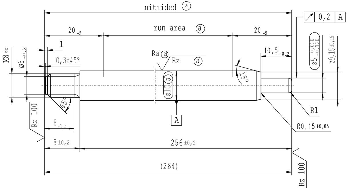
thread tolerances acc. to DIN ISO 965-3
