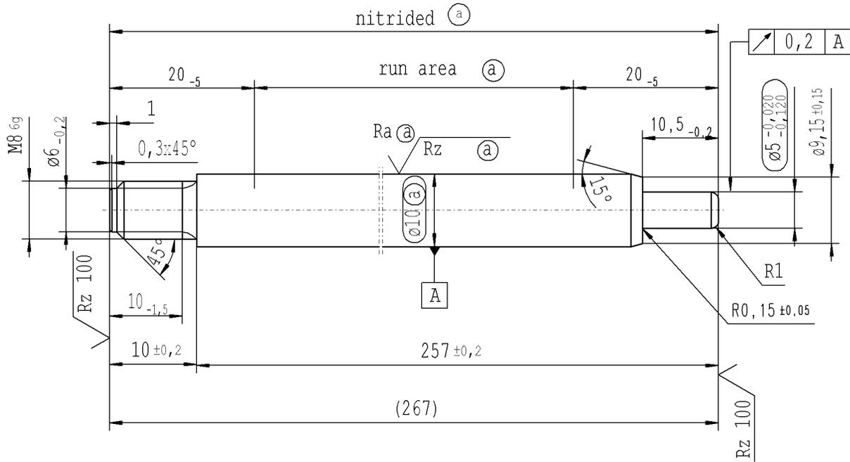
thread tolerances acc. to DIN ISO 965-3
