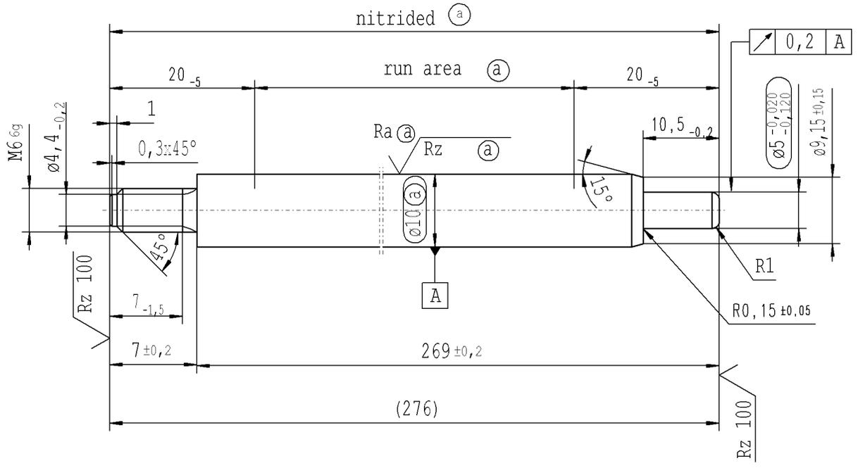
thread tolerances acc. to DIN ISO 965-3
