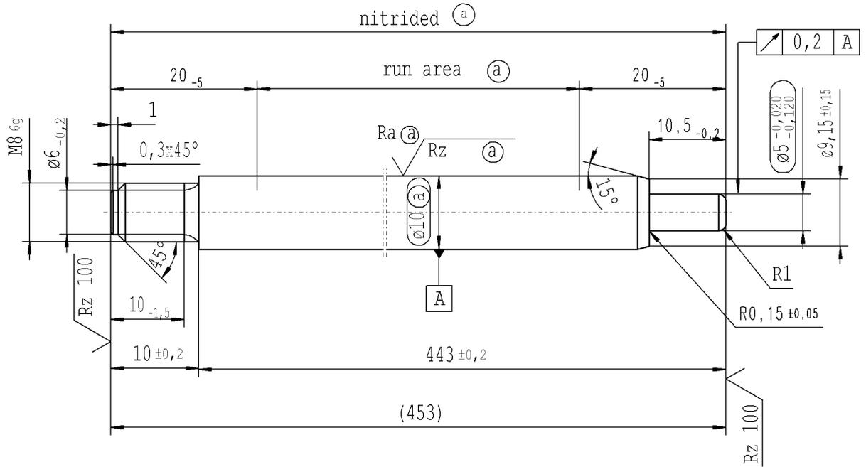
thread tolerances acc. to DIN ISO 965-3
