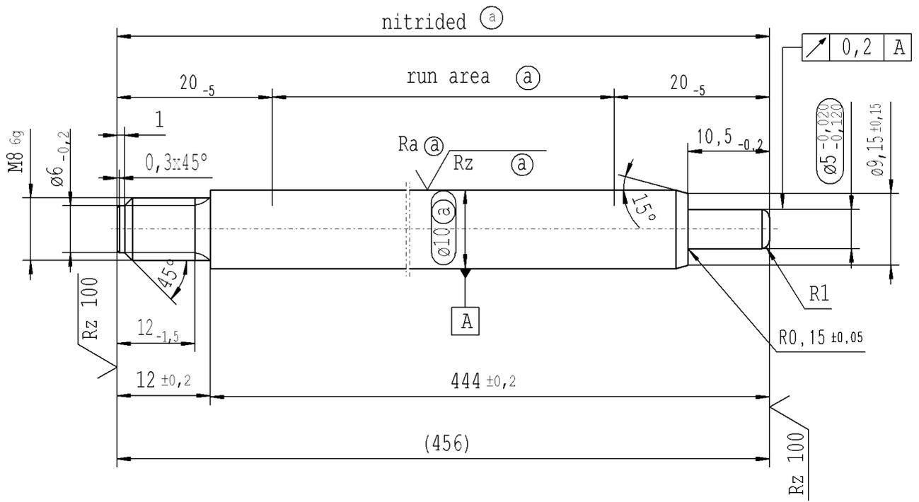
thread tolerances acc. to DIN ISO 965-3
