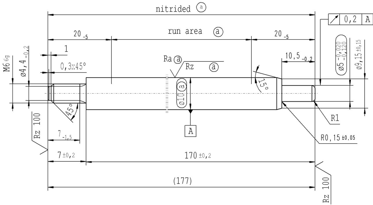
thread tolerances acc. to DIN ISO 965-3
