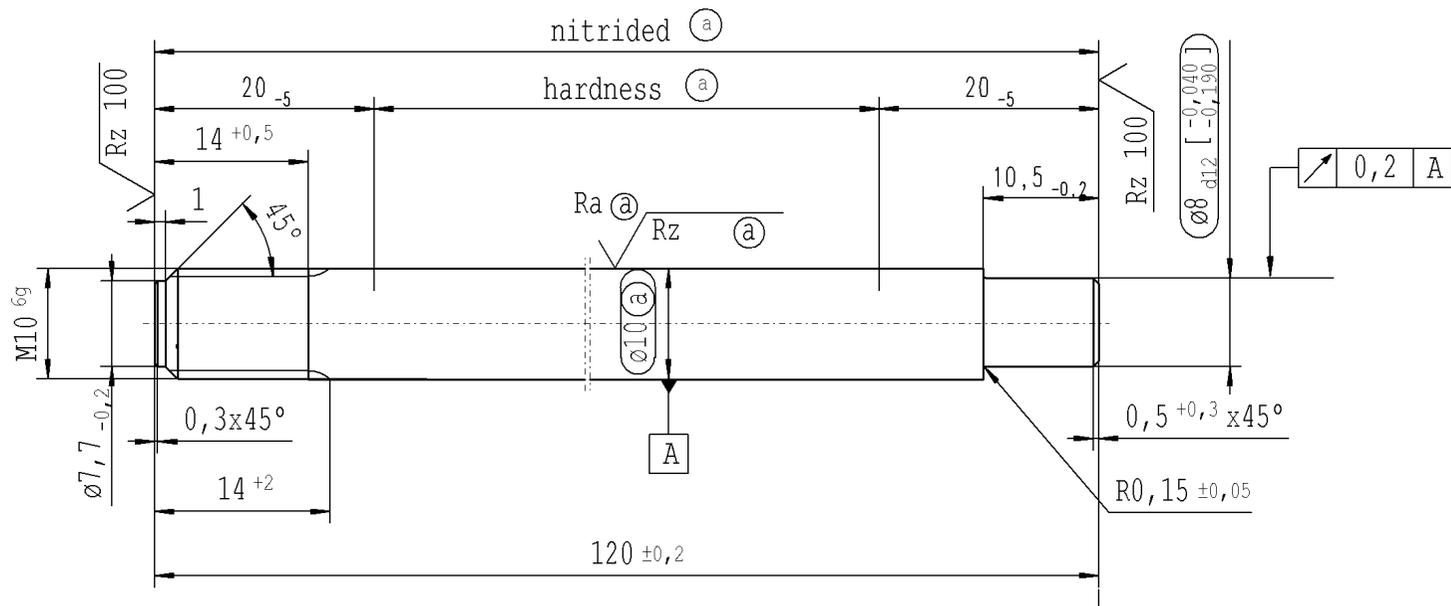
thread tolerances acc. to DIN ISO 965-3
