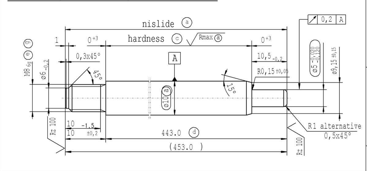
version 2 (only external production) \* material: 1.1193 S45C JISG 4051, for ZS-RO alt. 183844 (C35EC)
